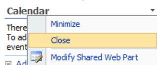
Figure 5.4 When you close a Web Part it is placed in the Closed Web Parts Gallery.
